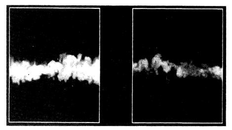
Fig. 8 Product formation end-view Mie scattering images for  $M_c = 0.28$ , x = 18 cm: a) (left) cut through vortex core; b) (right) cut through braid.
