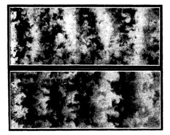
Fig. 7 Plan-view Mie scattering for  $M_c = 0.28$ , x = 15-30 cm (flow is from left to right): a) (upper) product formation method; b) (lower) passive scalar method.
