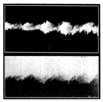
Fig. 6 Side-view Mie scattering for  $M_c = 0.28$ , x = 15-28 cm (flow is from left to right): a) (upper) product formation method; b) (lower) passive scalar method.
