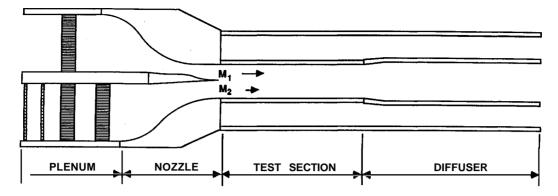
Fig. 1 Wind-tunnel schematic.
