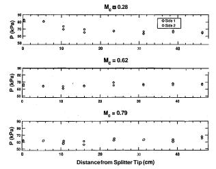
Fig. 3 Streamwise static pressure distributions: a)  $M_c = 0.28$ ; b)  $M_c = 0.62$ ; c)  $M_c = 0.79$ .
