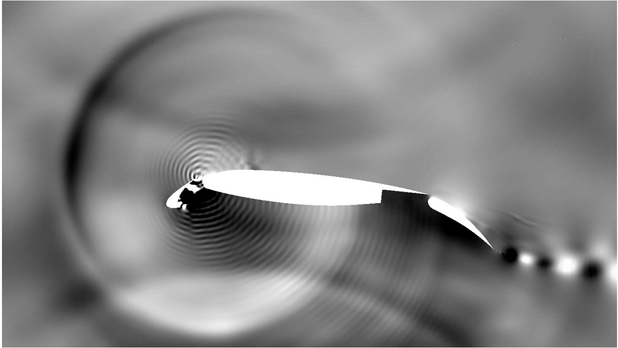
Figure 13: Instantaneous pressure fluctuation field at 4-degree AOA.
