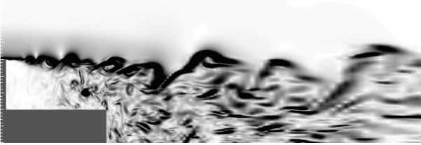
Figure 4. Instantaneous view of coherent structures educed using Q criterion (left view:DES ; right view: LES)
