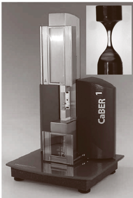
Fig. 9.54 CaBER® capillary breakup rheometer. Inset shows a closeup of a thinning fluid filament stretched in the instrument
