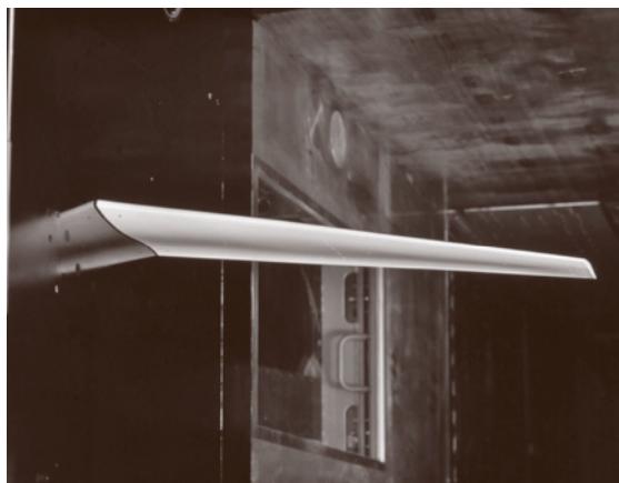
Fig. 8.83 Elastic wing models in the adaptive test section of a transonic wind tunnel
