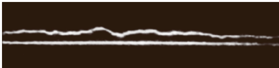
Fig. 5.158 Typical single-line RELIEF image pair taken in a turbulent free air jet with 0 \mu\text{s} (lower line), and 7 \mu\text{s} (upper line) time delay. The line is approximately 1.2 cm long (after [5.590], with permission of Cambridge Univ. Press)
