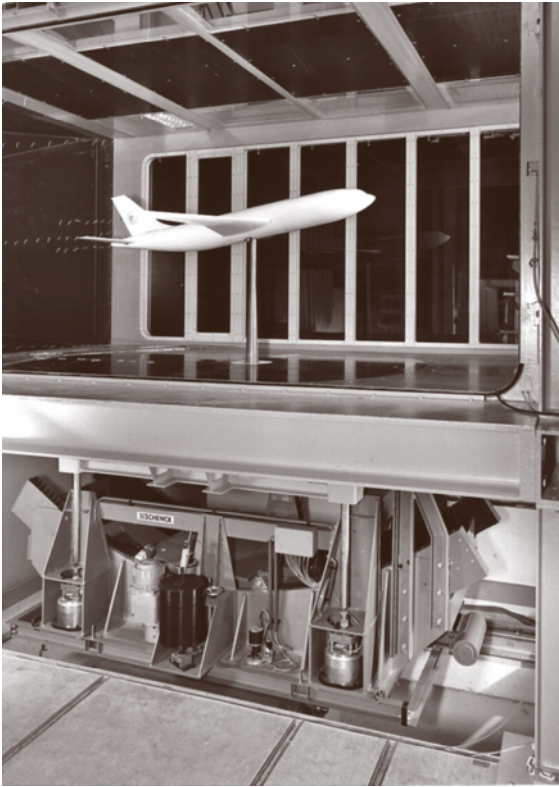
Fig. 8.3 External balance and support
