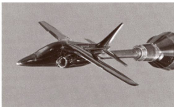
Fig. 8.13 Tail sting through engine nozzle
