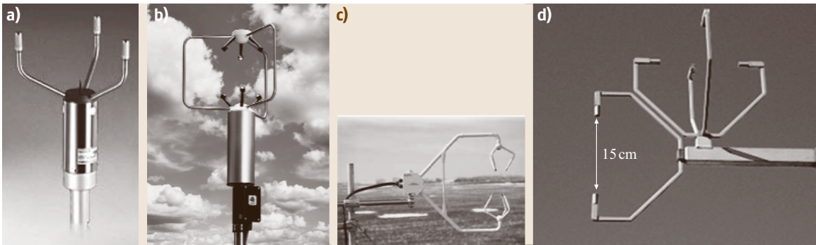
Fig. 5.221a–d Various sonic anemometer configurations: (a) 2-D sonic anemometer with vertical mounting base, (b) 3-D SAT with vertical mounting base, (c) 3-D SAT with horizontal mounting nonorthogonal pulse paths, (d) 3-D SAT with horizontal mounting and orthogonal pulse paths. Photographs are courtesy of (a) Vaisala, Inc. (b) RM Young Company, (c) Campbell Scientific, Inc. and (d) Applied Technologies, Inc.
