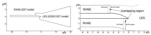
Figure 5: Layout of zonal RANS-LES simulation of hydrofoil trailing edge flow.
