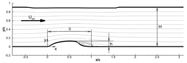
Figure 1: Schematic of the wall-mounted hump flow.
