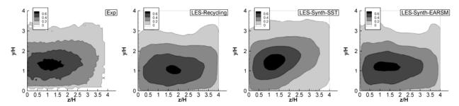
Figure 10: Comparison of averaged streamwise velocity fields at the exit plane of the diffuser (x/H=15).
