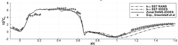
Figure 4: Wall friction comparison for the wall-mounted hump flow.
