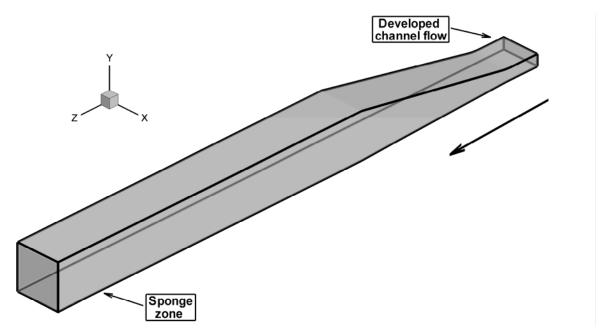
Figure 8: Schematic of the three-dimensional diffuser.
