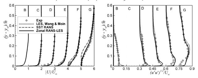
Figure 7: Comparison of averaged streamwise velocity and rms of streamwise velocity fluctuations profiles for hydrofoil trailing edge flow. Here  $y_w$  denotes y-coordinate of the wall.
