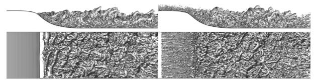
Figure 3:  $\lambda_2$  isosurfaces for wall-mounted hump flow. IDDES in the whole domain is on the left, zonal RANS-IDDES is on the right.
