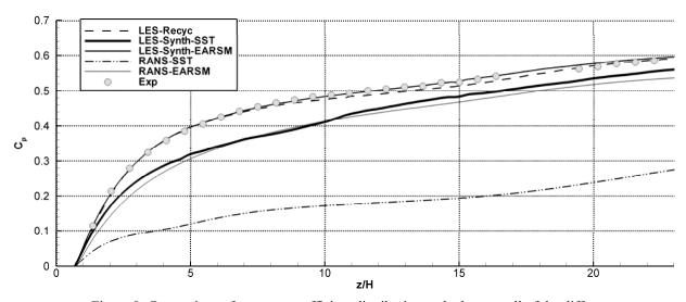
Figure 9: Comparison of pressure coefficient distribution at the lower wall of the diffuser
