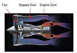
Figure 1: Turbofan engine<sup>1</sup>
