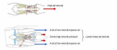
Figure 2: A turbojet and a high bypass ratio turbofan engine and their jet velocities<sup>2</sup>
