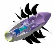
Figure 5: Pusher configuration<sup>5</sup>
